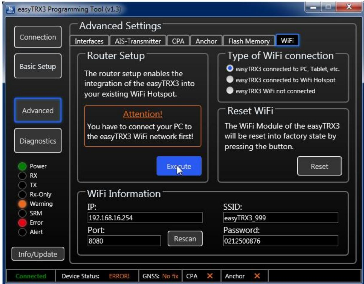
Figure: 38 WiFi connected to PC, Tablet, etc. (1)
