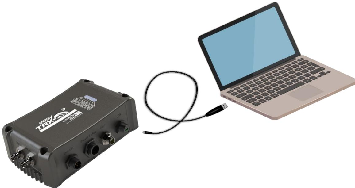
Figure: 8 Base connection by USB for programming
